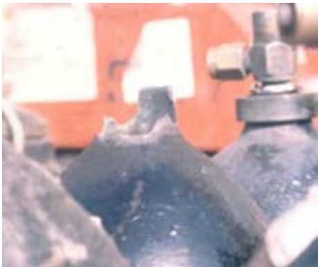
Hydrocarbon-based cylinder valve fire
